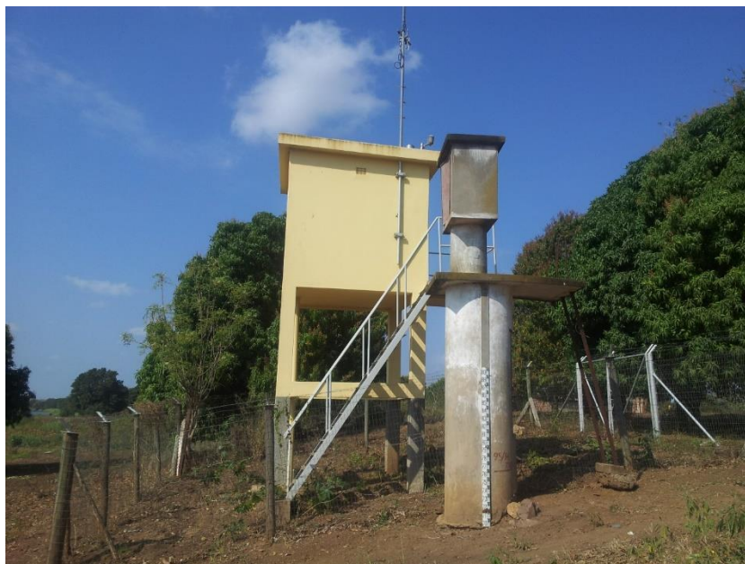
Figure 16 Hydrometric scale as an early warning sensor in Chókwe
