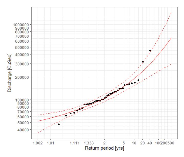
Part A - Flood Frequency Curve of Kabul River (Nowshera) - based on daily flow data from 1982 to 2022
